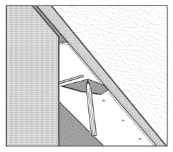
With the reflector cut out left and frontward, align the steam deflector with the front edge of the counter. Trace the outline of the reflector onto the underside of the counter with a pencil.
